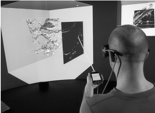
Fig. 6. Using the PDA as a virtual laser pointer for object selection
