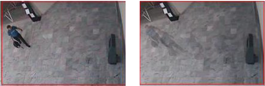
Fig. 1c. Temporal Magic Lens detail from Fig 1a. Left: Defining the temporal magic lens. Right: Seeing through the temporal magic lens; the ghosting gives a preview of “future” events. The effect is more evident from the actual motion of the video in the prototype system when viewed interactively, than in the static images shown here.
