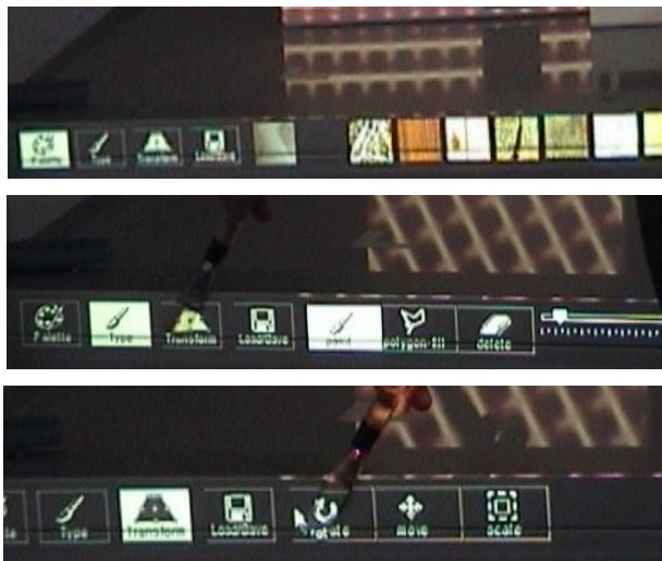
Fig. 2. From above: a) the menu item palette displays all the textures to choose from. b) the menu item “type” with brush, polygon fill, delete, and a bar to adjust the size. c) “transform” with the possibility to rotate, move, and scale.
