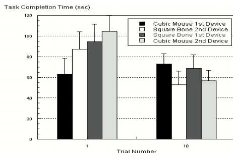
Fig. 5. Mean task completion times (TCTs) and standard errors for the CubicMouse and the SquareBone obtained in trials 1 and 10 separately for the group beginning with the CubicMouse and the one beginning with the SquareBone
