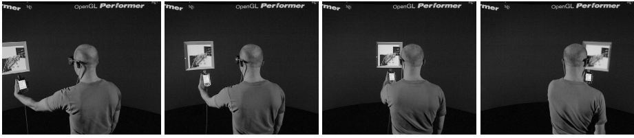
Fig. 7. Large object motion with Scaled Grab: Note alignment between PDA and virtual object
