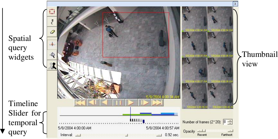
Fig. 1a. The Temporal Magic Lens includes four basic widgets: video player with spatial query widgets (upper left quadrant), timeline sliders to control the temporal query (bottom left corner), thumbnail views for drill down (right-hand side), and compositing/rendering techniques (inset of video player, and below in Figure 1c).
