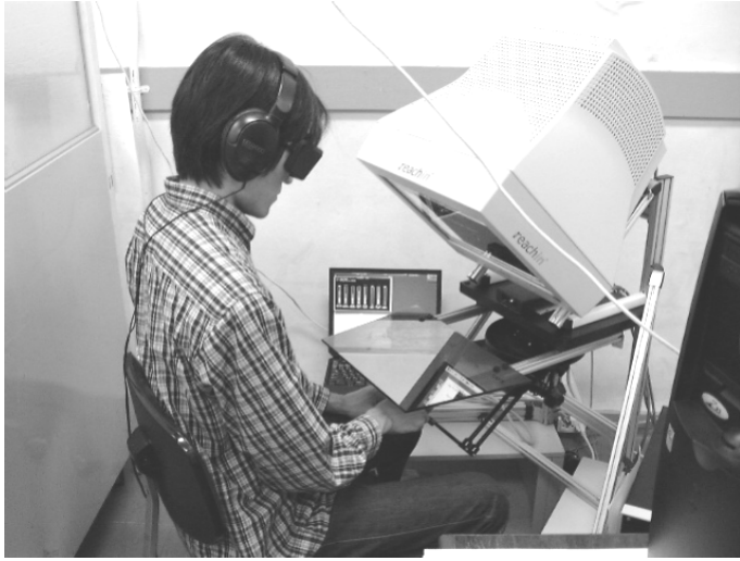
Fig. 1. Experimental environment with PHANToM and Reachin Display
