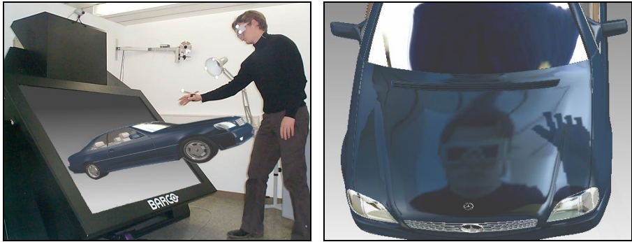
Fig. 2. Responsive workbench environment with tracked head, hand, and floor lamp (left). Reflections and shadows on the engine hood from the user's point of view (right).
